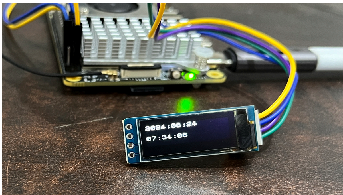
Fig. 5.24: Date & Time on 128x32 OLED
