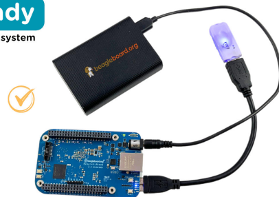
Fig. 2.9: USB OTG to connect USB gadgets to BeagleV Ahead board
